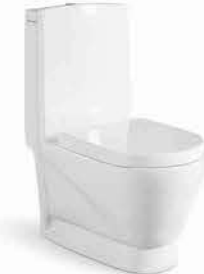
8023 Washdown one-piece toilet Size:710x375x870 mm P-trap,180mm roughing-in S-trap,250mm roughing-in
