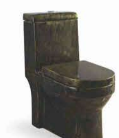
9008 Washdown one-piece toilet Size:740x410x760 mm P-trap,180mm roughing-in S-trap,250mm roughing-in
