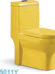
5011Y Siphonic/Washdown one-piece toilet Size:720x370x810 mm P-trap,180mm roughing-in S-trap,250/300x400mm roughing-in
