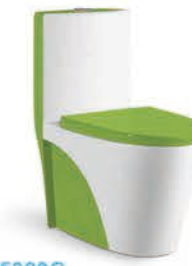
5008G Siphonic/Washdown one-piece toilet Size:685x385x765 mm P-trap,180mm roughing-in S-trap,300/400mm roughing-in
