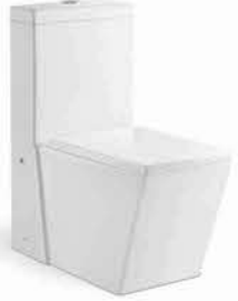
8037 Washdown one-piece toilet Size:680x390x820 mm P-trap,180mm roughing-in S-trap,250mm roughing-in
