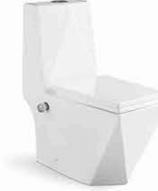
F-8001 Washdown one-piece toilet Size:685x380x820 mm P-trap,180mm roughing-in S-trap,250mm roughing-in
