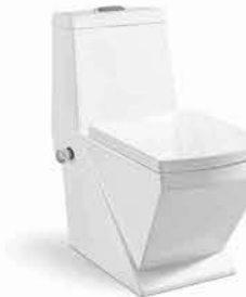
F-8007 Washdown one-piece toilet Size:720x380x750 mm P-trap,180mm roughing-in S-trap,250mm roughing-in
