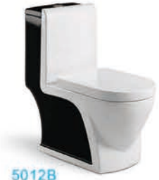
5012B Siphonic/Washdown one-piece toilet Size:720x370x780 mm P-trap,180mm roughing-in S-trap,250/300x400mm roughing-in
